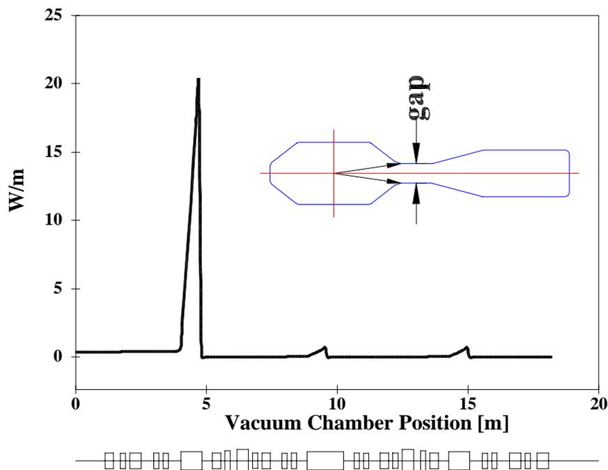
Figure f26\_e: **Power Distribution of the Vacuum Chamber at 2.4 GeV and 400 mA for a Magnet Section**
