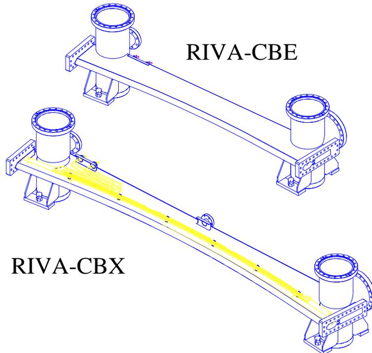
Figure f26\_c: **Dipole chamber RIVA-CBE for dipole BE and RIVA-CBX for dipole BX**
