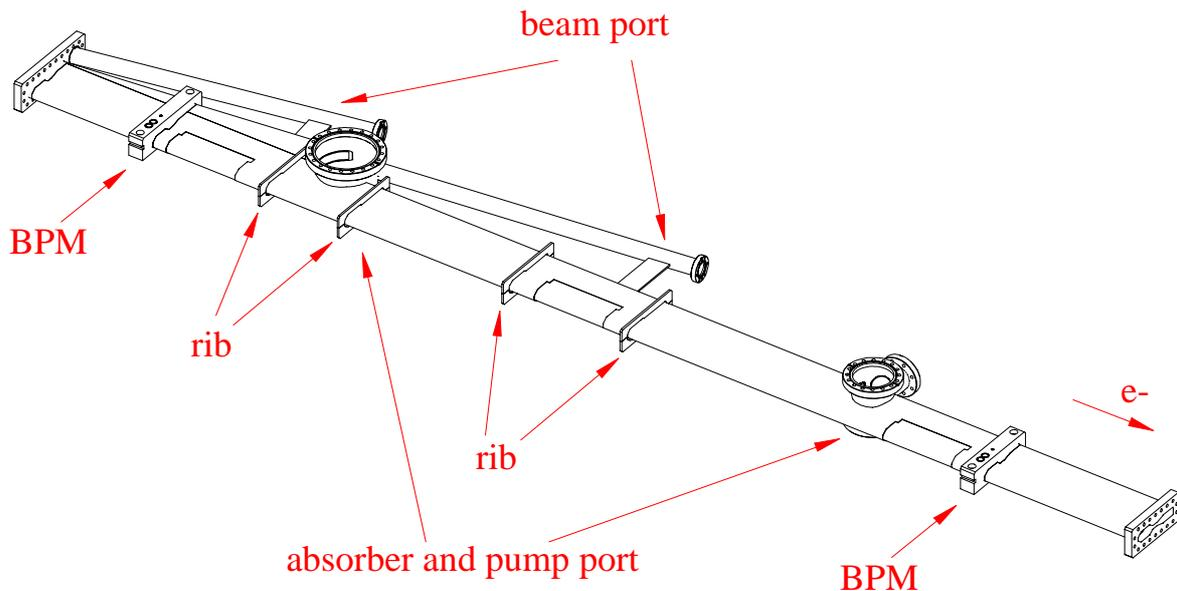
Figure f26\_h: **Quadrupole chamber RIVA-CGM2**
