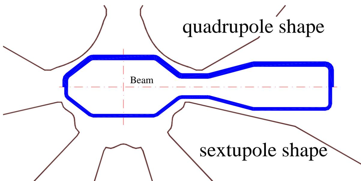
Figure f26\_b: Chamber cross section with quadrupole and sextupole shape
