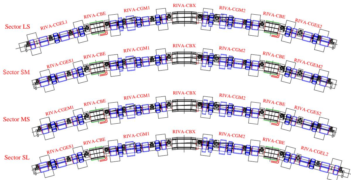
Figure f26\_a: **Storage ring cells LS, SM, MS, and SL with vacuum system**
