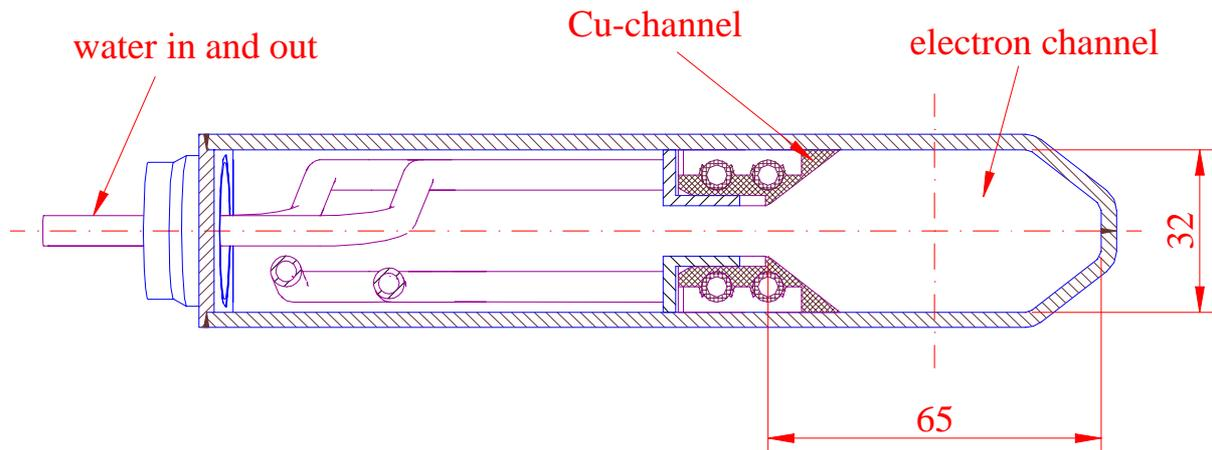
Figure f26\_f: Dipole chamber cross section
