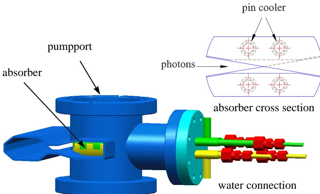
Figure f26\_d: **Photon Absorber in the Quadrupole Chamber**
