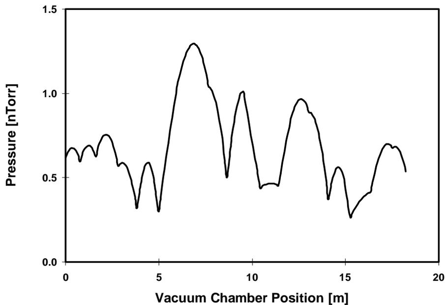
Figure f26\_i: CO Pressure Distribution for a Magnet Section (2.4 GeV, 400 mA, 100 Ah)
