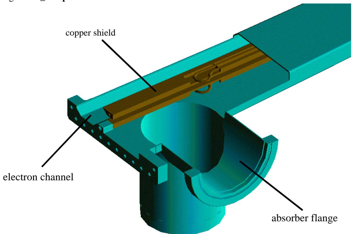
Figure f26\_g: Copper shield in the Dipole chamber
