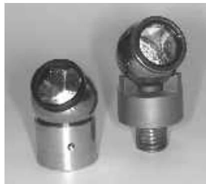
Fig. f711 d Sphere mounted glass and air reflector
