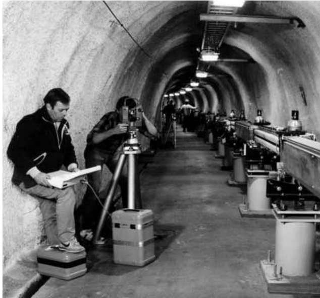
Fig. f711 a Forced Centered Set-up at SLAC
