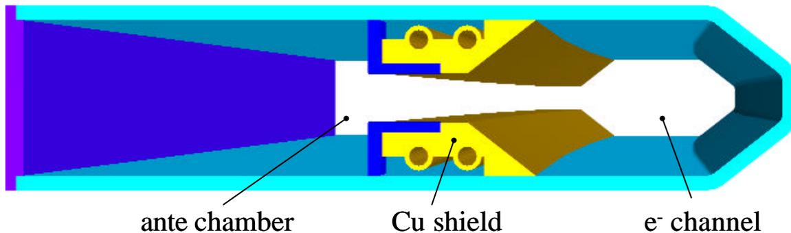
Fig. 3 Dipole chamber with water-cooled copper shield
