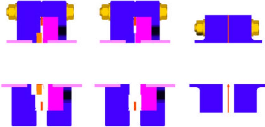
Fig. 4a CF Flange with RF bridge
