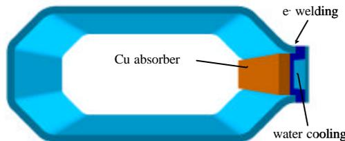
Fig. 2a Vacuum Chamber with indirectly cooled Cu absorber (ANKA, BESSY II)
