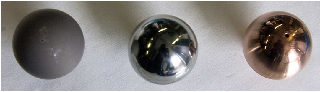
Figure 3: Three anodes used for HV testing, Ti on the left (grey black colour, after vacuum firing), Mo in the center and Cu on the right. Pictures taken after HV testing. Damages can be seen on the Ti electrodes
