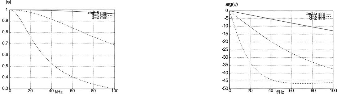
Figure 3: Absolute value and complex phase shift of the magnetic flux versus frequency. Sheet thickness  $d = 0.5, 1, 2$ mm. Material parameters:  $\mu = 3500$ ,  $\kappa = 4 \cdot 10^6$
