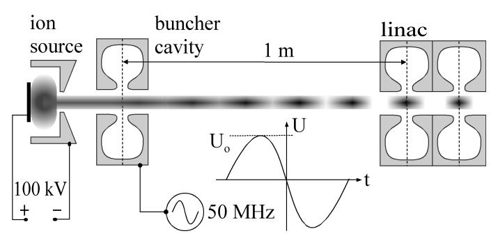
Question: What's the required voltage amplitude  $U_o$  of the buncher cavity?
