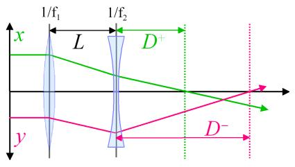
Abbreviations for convenience:  $g = \frac{1}{f_1}$ ,  $f = \frac{1}{f_2}$ Calculate the transfermatrix by multiplication of thin-lens- and drift-matrices:
